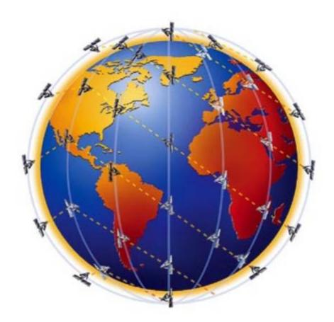
The Iridium system is the only communications system providing true global communications coverage of every ocean, all land areas, and the Poles. The network blankets the Earth, enabling two-way communications for devices installed in remote areas.
