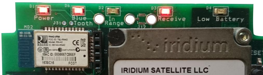
These lights are on the top of the circuit board and can be seen without opening the enclosure.
